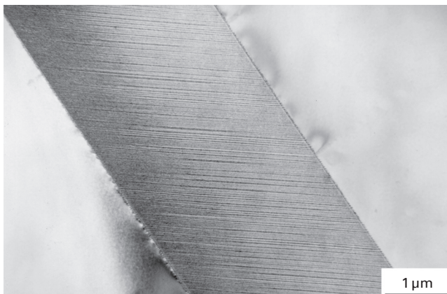
2.14 Transmission electron micrograph of thin plate martensite in Fe-30%Ni-0.39%C alloy ( M_s = 133 K) (Maki and Tamura, 1986).
