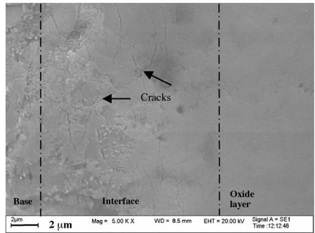
Fig. 9. SEM micrograph at the edge of SIMS crater. Laser parameter: power 10 W, scanning speed 500 mm/s, two scan passes.
