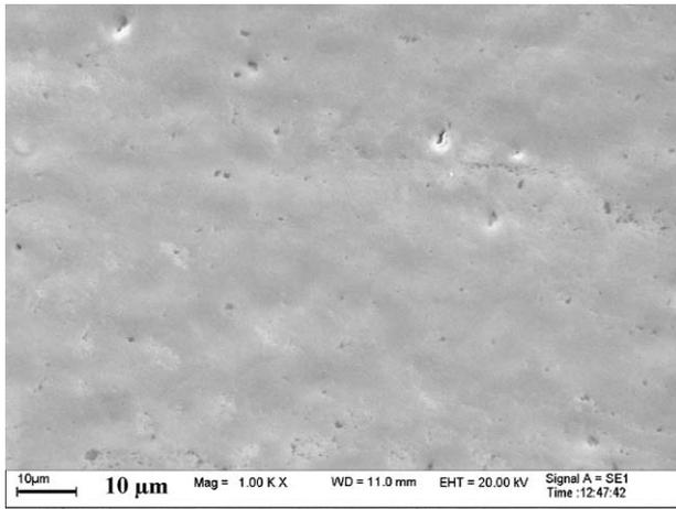
**Fig. 5.** SEM micrograph of the sample after two laser scan passes at power of 10 W and scanning speed of 500 mm/s.
