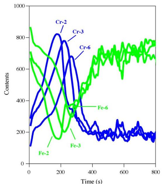
Fig. 11. Cr:Fe ratio in the laser-induced oxide layer. Laser parameters: power 10 W, scanning speed 500 mm/s. The numbers denote the number of laser scan passes.
