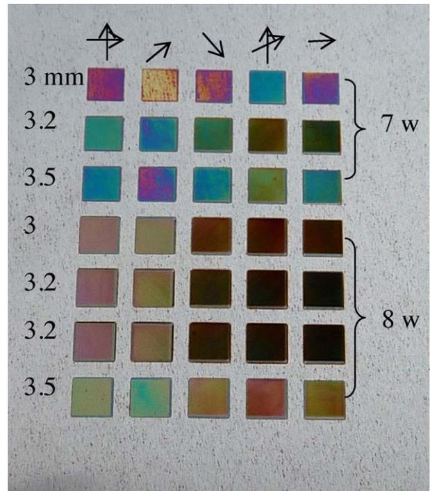
Fig. 1. Laser produced colors on stainless steel at various processing parameters.
