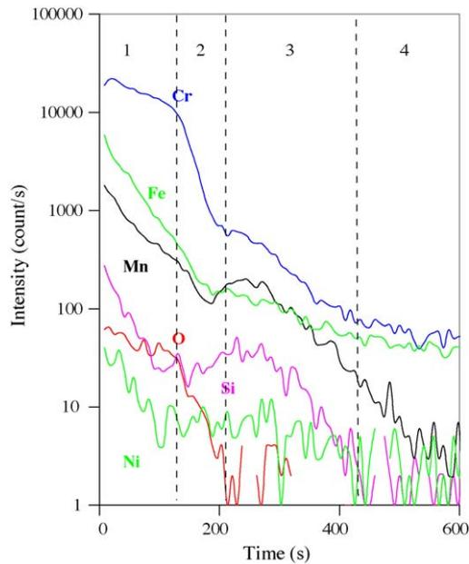
Fig. 7. TOF-SIMS depth profiles of the sample after one laser scan pass. Laser parameters: power 10 W, scanning speed 400 mm/s.
