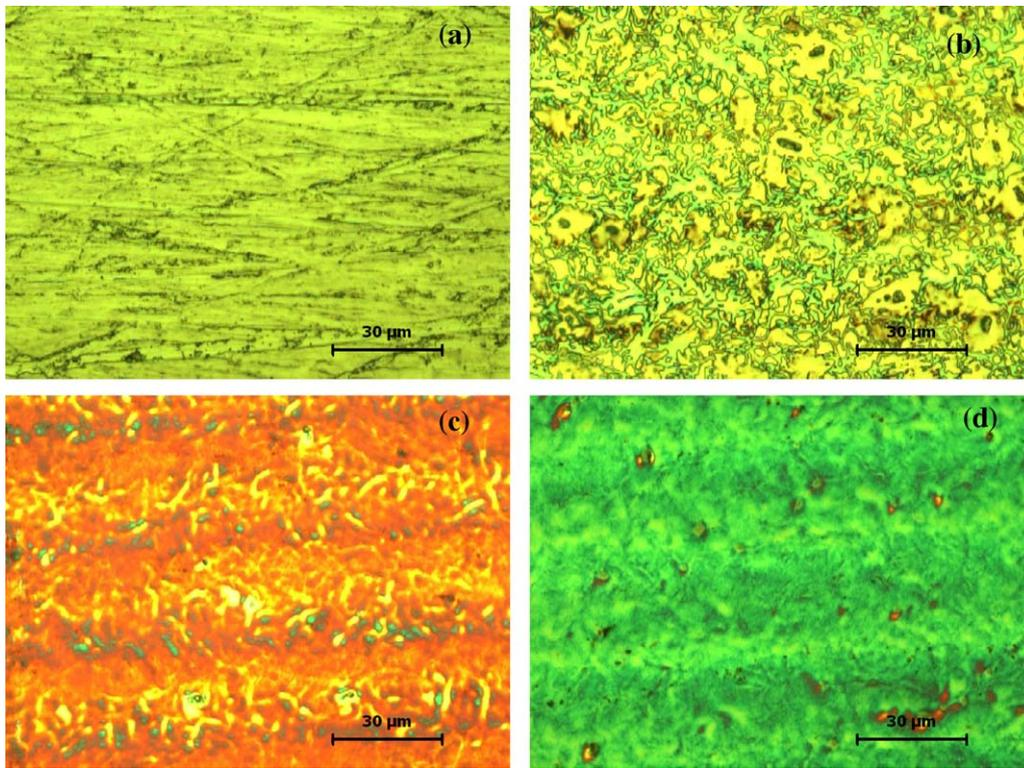
**Fig. 2.** Optical micrographs of the samples for (a) as-received, and laser scans at (b) one pass, (c) two passes, and (d) three passes. Laser parameters: power 10 W, scanning speed 500 mm/s.
