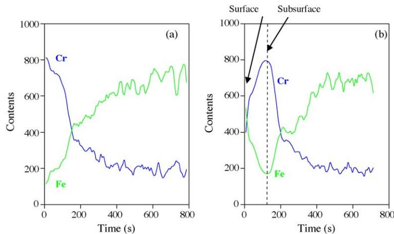
Fig. 10. Cr:Fe ratio in the laser-induced oxide layer. One scan pass at a scanning speed of (a) 500 mm/s and (b) 400 mm/s. Laser parameters: power 10 W.
