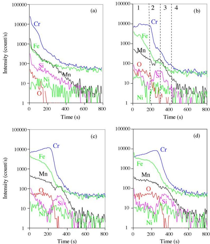
**Fig. 6.** TOF-SIMS depth profiles of the samples after laser scans of (a) one passes, (b) two passes, (c) three passes, and (d) six passes. The numbers on (b) denote the sub-layers. Laser parameters: power 10 W, scanning speed 500 mm/s.
