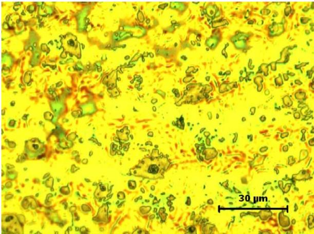
**Fig. 3.** Optical micrograph of the sample after one laser scan pass at power 10 W and scanning speed of 400 mm/s.
