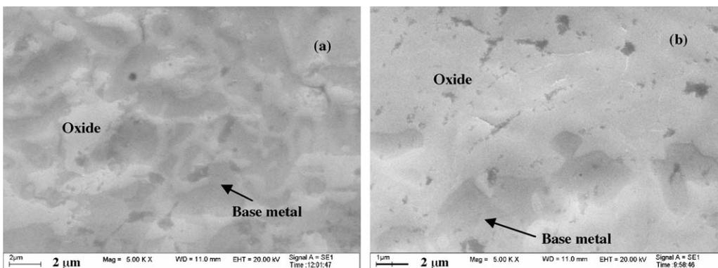
**Fig. 4.** SEM micrographs of the samples after one laser scan pass at power 10 W and scanning speed of (a) 500 mm/s and (b) 400 mm/s.
