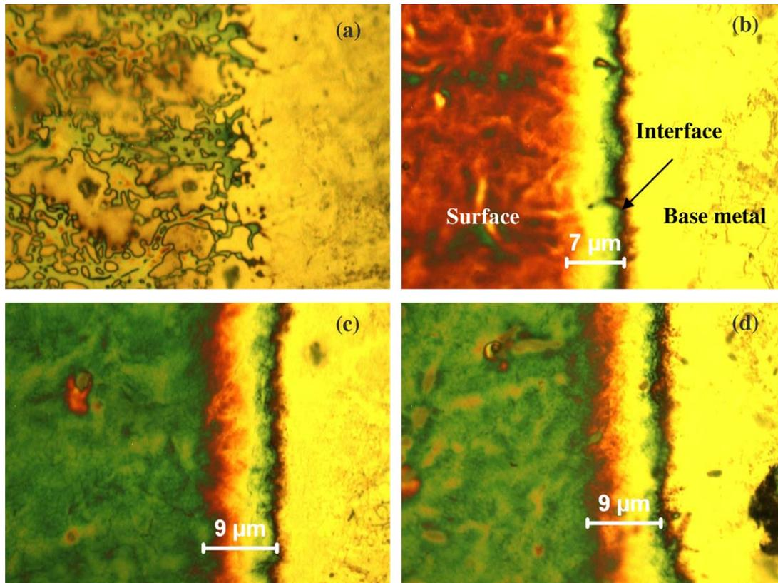
Fig. 8. Optical micrographs of the edges of SIMS craters. Laser scan passes were (a) one, (b) two, (c) three, and (d) six. The laser parameters: power 10 W and scanning speed 500 mm/s.
