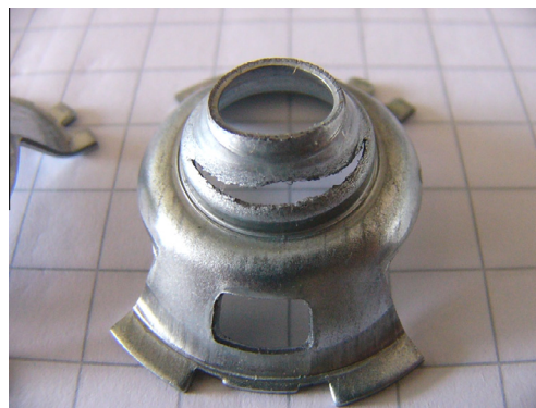
Fig. 3. Fracture of the wall. The fracture in direction of rolling of material shows worse workability of sheet in transversal direction, Steel 2: The grid is 1 \times 1 cm.
