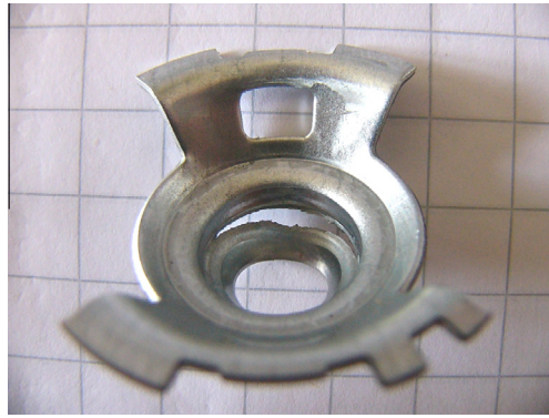
Fig. 4. Internal part of the housing with fracture, Steel 2: The grid is 1 \times 1 cm.
