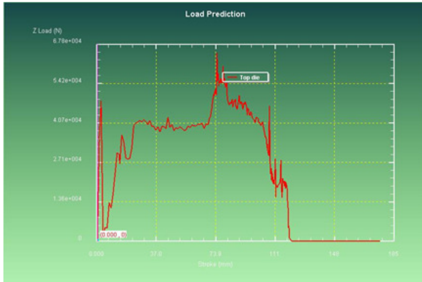
Figure 3.4.1 Coefficient of friction=0.12 having shear angle=120°
