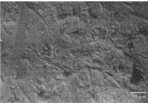
Fig. 9. Surface morphology of the VPS coating after 500 revolutions with the 100 μm abrasive.
