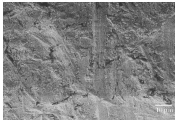
Fig. 7. Surface morphology of the APS1 coating after 500 revolutions with the 100 μm abrasive.
