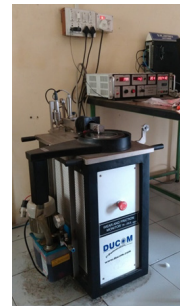
Fig. 2. Pin-on-disc wear testing apparatus.
