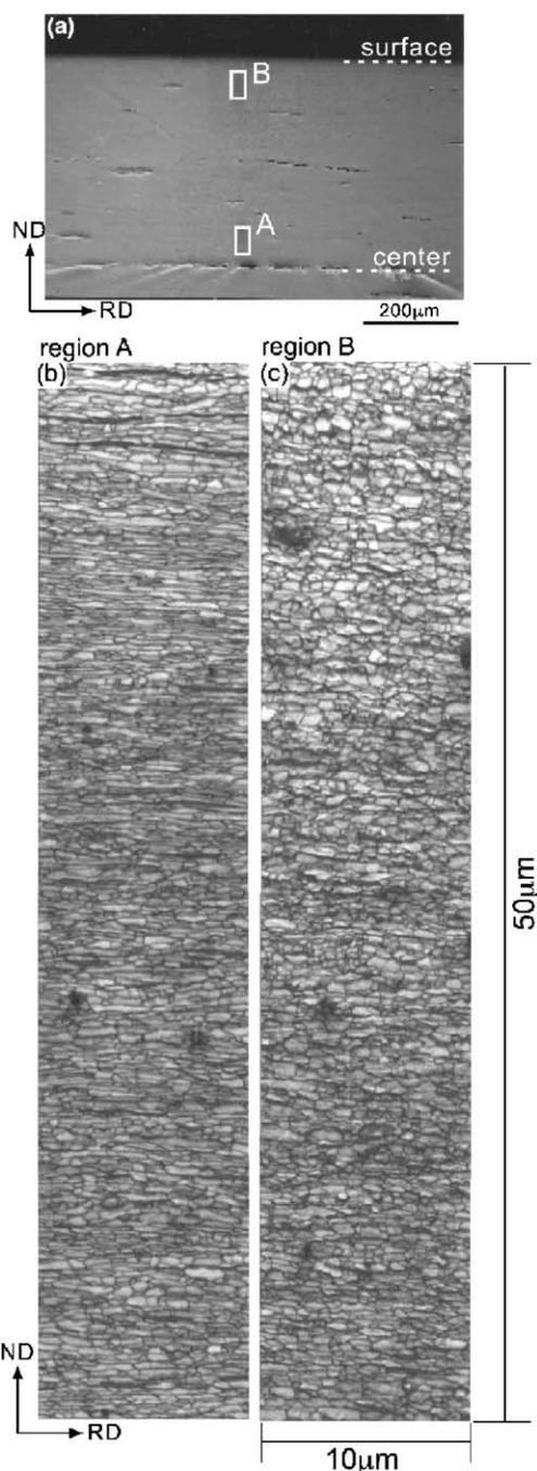
Fig. 2. SEM micrograph (a) of the ARB processed IF steel and IQ maps of the regions A (b) and B (c) obtained by EBSD measurement in FE-SEM.
