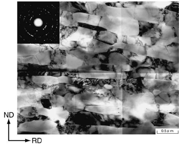
Fig. 1. TEM micrograph and corresponding SAD pattern of the IF steel sheet ARB processed by five cycles ( $\epsilon = 4.0$ ) at 773 K. Observed from TD near the thickness center of the sheet.
