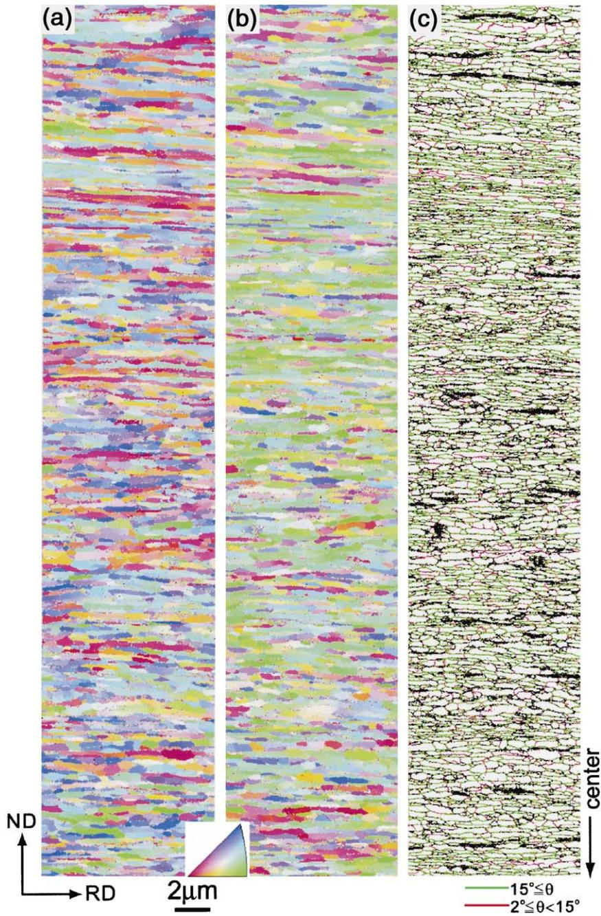
Fig. 3. Orientation imaging microstructures of the region A (near center) obtained by EBSD measurement. (a) ND orientation color map, (b) RD orientation color map, (c) boundary misorientation map.
