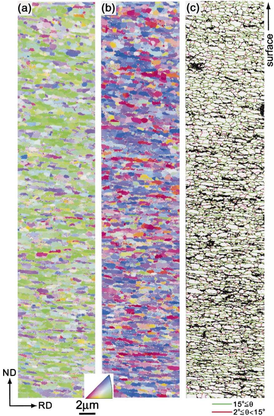
Fig. 4. Orientation imaging microstructures of the region B (near surface) obtained by EBSD measurement. (a) ND orientation color map, (b) RD orientation color map, (c) boundary misorientation map.
