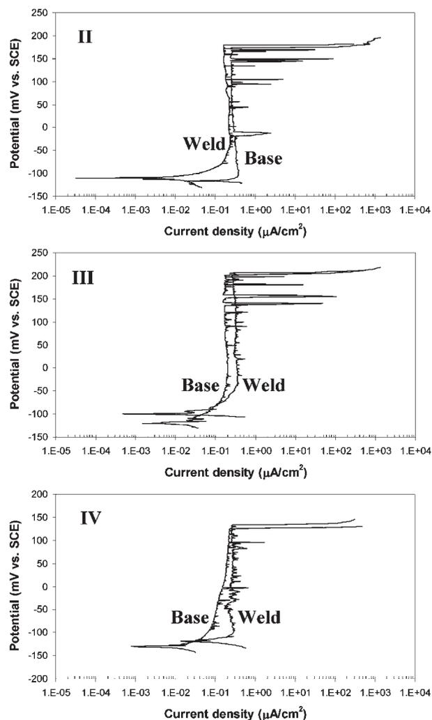
**7 Potentiodynamic polarisation curve for individual base and weld regions of repair welded 17-4PH stainless steel in II, III and IV, immersed in 3.5%NaCl solution. Scan rate was 3 mV min<sup>-1</sup>**
