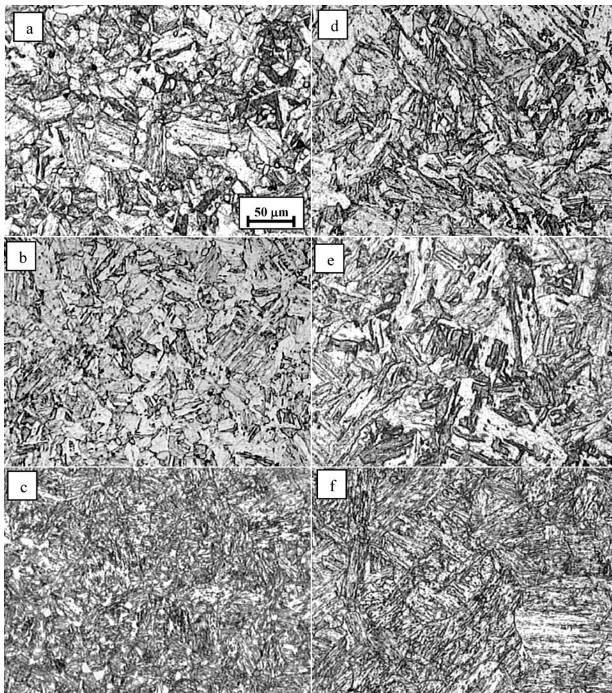
3 Optical images of *a–c* base and *d–f* weld regions of GTA welded 17-4PH in three different PWHT conditions (II, III and IV) respectively
