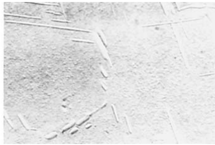
Fig. 3 Typical operating microstructures of representative superalloys. (a) Cast cobalt-base alloy. 250 \times . (b) Cast nickel-base alloy. 100 \times (c) Wrought (left, 3300 \times ) and cast (right, 5000 \times ) nickel-base alloys. (d) Two wrought iron-nickel-base alloys (left, 17,000 \times ; right, 3300 \times ). Note script carbides in (a) and (b) as well as eutectic carbide-cobalt grain-boundary structures in (a), spheroidal and cuboidal \gamma' as well as grain-boundary carbides in (c), and spheroidal \gamma' as well as grain-boundary and intragranular \delta phase in (d). \gamma'' not obvious but present in (d) (right).
