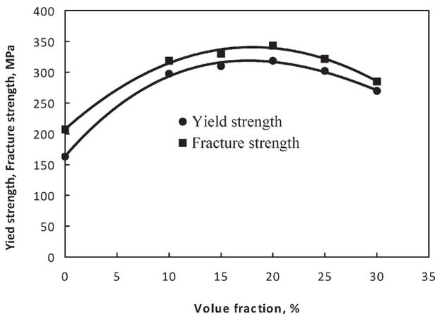
11 Variations of yield strength and fracture strength with volume fraction of SiC
