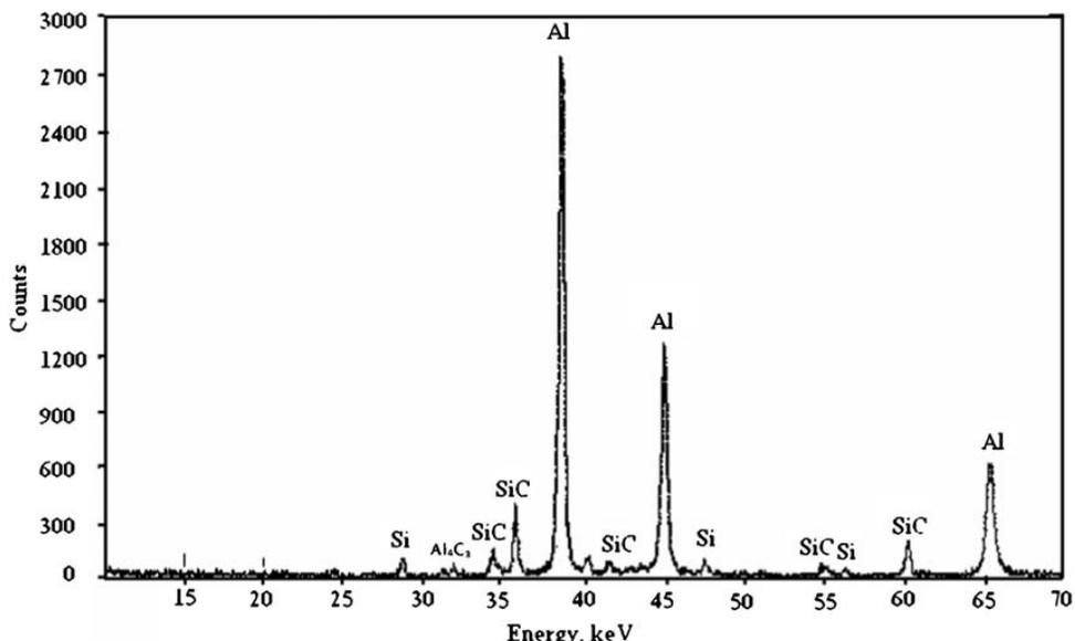
7 X-ray diffractogram of heat treated 7072 Al/SiC<sub>p</sub> (V<sub>f</sub>=20%) composite
