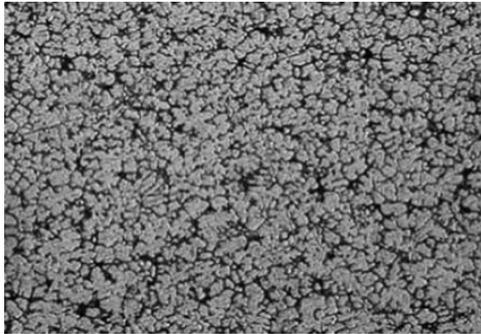
3 Microstructure of heat treated 7072 Al alloy
