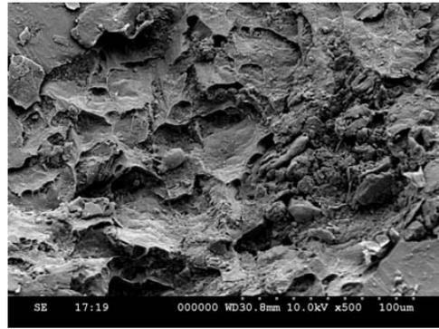
15 Image (SEM) of fracture surface of as cast tensile sample ( $V_f=30\%$ )
