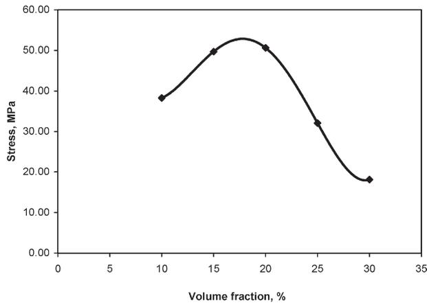
12 Variation of strain hardening with volume fraction of SiC
