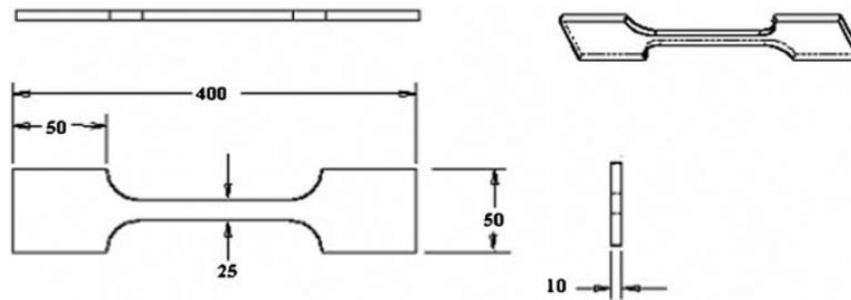
2 Tensile specimen: all dimensions are in millimetres
