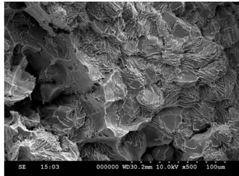
16 Image (SEM) of fracture surface of heat treated fatigue sample ( $V_f=30\%$ )
