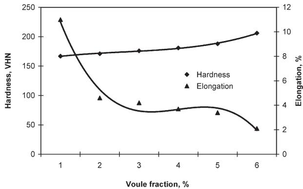
13 Variations of ductility and hardness with volume fraction of SiC particles
