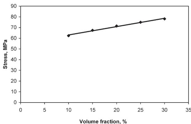
14 Variation of strain hardening with volume fraction of SiC
