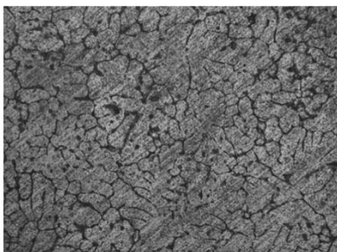
4 Microstructure of 7072/SiC<sub>p</sub> as cast composite ( $V_f=20\%$ )
