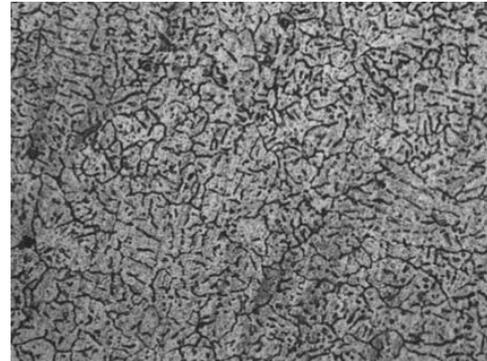
5 Microstructure of 7072/SiC<sub>p</sub> heat treated composite ( $V_f=20\%$ )
