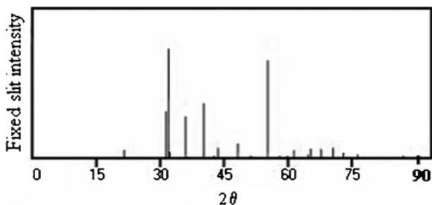
8 X-ray analysis to recognise second phase of Al<sub>4</sub>C<sub>3</sub>
