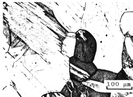
FIG. 5 Microstructure of the Cu-11%Al - 6.9%Mn alloy. Note the thick heavily twinned martensitic plates in this partially martensitic at room temperature alloy, which has a higher aluminium content than that of Fig. 4.
