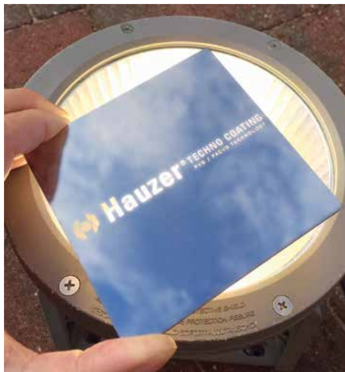
Figure 3. Example of translucent plate with thin Cr coating held above a lamp.
