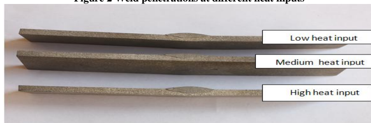
Figure 2 Weld penetrations at different heat inputs
